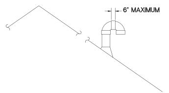
Figure 26 – Vertical Rooftop Air Inlet
